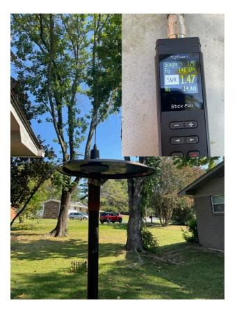
2 meter antenna mounted on pizza pan on steel post.
